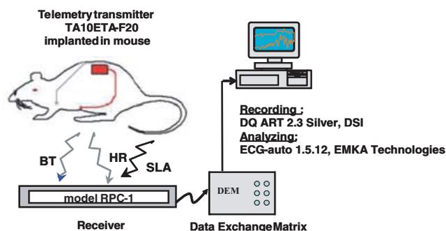
**Figure 1.** Heart rate variability set-up
