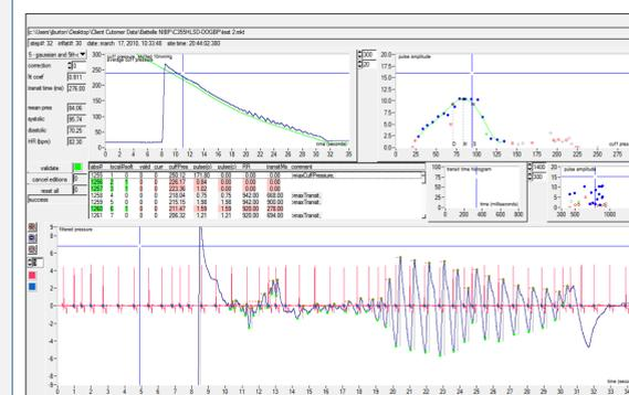
Figure 5. NIBP Telemetry – EMKA Screenshot of Cuff Pressure (upper left), a Plot of Cuff Pressure Plotted Against Pulse Amplitude (upper right), and Filtered Pressure With ECG Overlay for a Single Animal Treated With Prazosin
